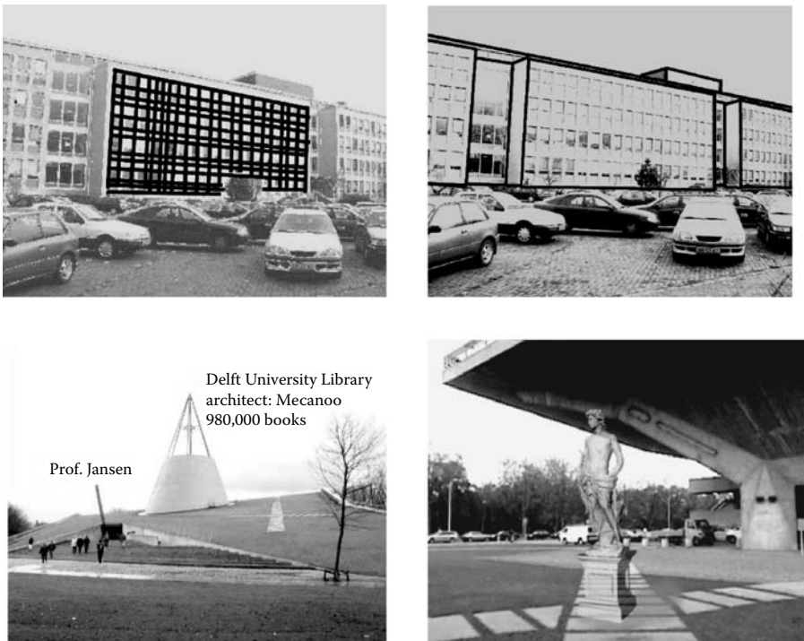
FIGURE 1.8 Ubicom example of outdoor augmented reality (top row: matching features from the 3D database with the real world image for correct positioning and orientation; lower left: adding textual information to objects in the real world image; lower right: adding designed objects to the real-world image).
