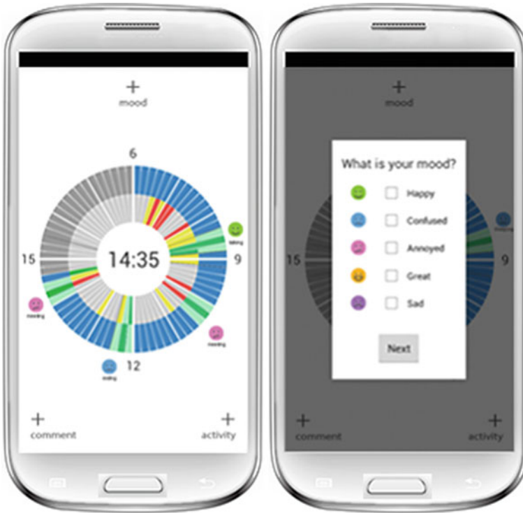
Fig. 14.5 ESTHER 1.3: Left ; the application showing the state of 3/4 of a day gone, the planned activities ( outer green strips ), the actual physical activity progress ( inner red, yellow and green strips ) and the mood/activity reported ( outer emoticons ). Right ; the mood self-reporting menu
