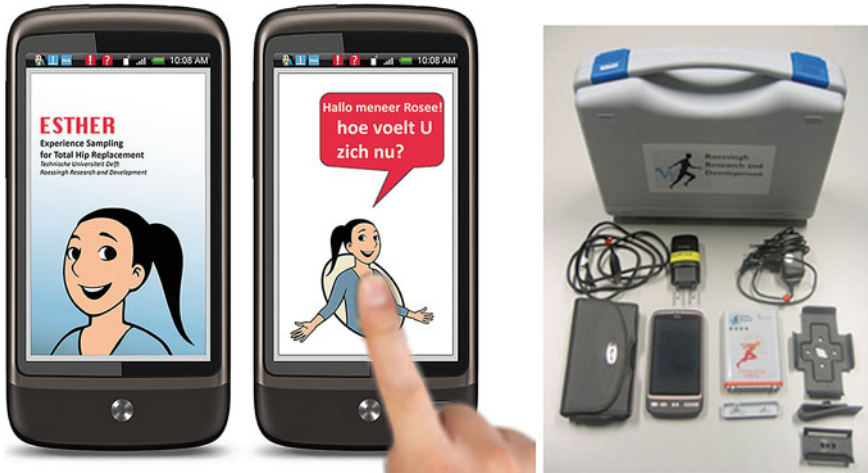
Fig. 14.4 ESTHER 1.2: Left , the application running on an Android phone; Right , the complete kit including the sensor node, the mobile phone, chargers and belt holders
