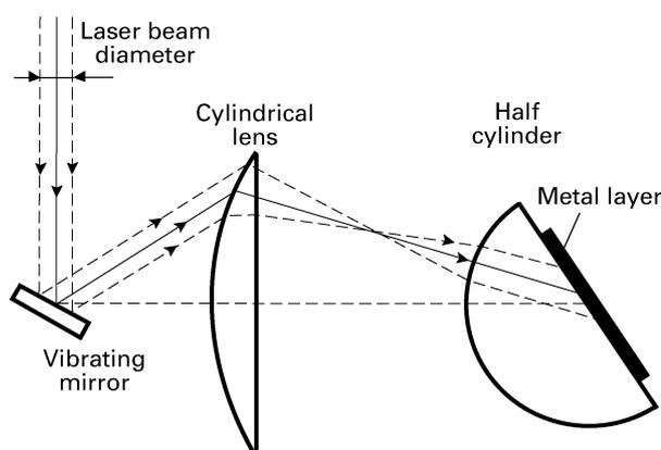
**Figure 6** Vibrating mirror setup. a: vibrating mirror; b: cylindrical lens. Reproduced with permission from Lenferink ATM (1991) *Sensors and Actuators B (Chemical)* 3: 261. Copyright 1991, with kind permission from Elsevier Science Ltd, The Boulevard, Langford Lane, Kidlington, OX5 1GB, UK.
