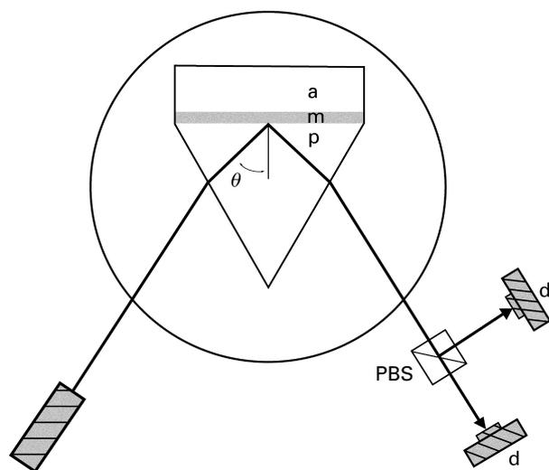
**Figure 3** Rotation stage SPR setup. d: detectors; PBS; polarizing beamsplitter.
