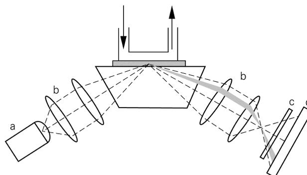
**Figure 4** Use of focused beam. a: laser diode; b: focusing optics; c: neutral density filter; d: diode array. A flow cuvette is placed on top of the metal layer. Reproduced with permission from Sjölander S (1991) *Analytical Chemistry* **63**: 2338. © American Chemical Society.
