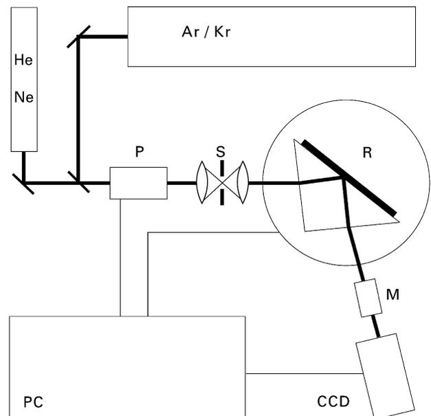
**Figure 10** SPR microscope setup. P: Pockels cell; S: spatial filter; R: rotation stage; M: objective; CCD: video camera.
