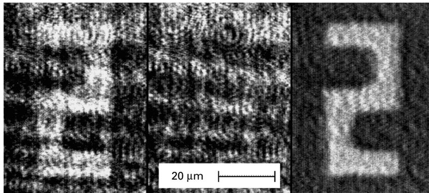
**Figure 11** Improvement of image quality by dividing s- and p-polarized responses. From left to right: p response; s response; p/s response.
