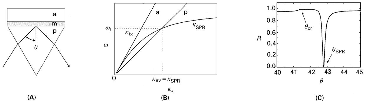
**Figure 1** The SPR experiment. (A) a metal layer m is sandwiched between two dielectric media a and p. The direction x is defined parallel to the layer structure; (B) dispersion relation of SPs; see text; (C) a typical SPR curve when medium a has a refractive index  $n_a = 1$ . The angle  $\theta_{cr}$  corresponds to the critical angle for the a/p interface.
