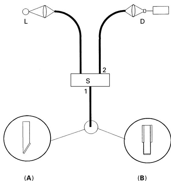
**Figure 7** Use of fibre optics. L: light source; D: detector; S: fibre splitter/combiner; 1, 2: output ports. (A): single mode fibre; (B): multimode fibre (cf. text).
