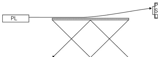
**Figure 5** Basic photothermal detection setup. The position of the deflected beam of a probe laser PL is measured by a position-sensitive detector PSD.
