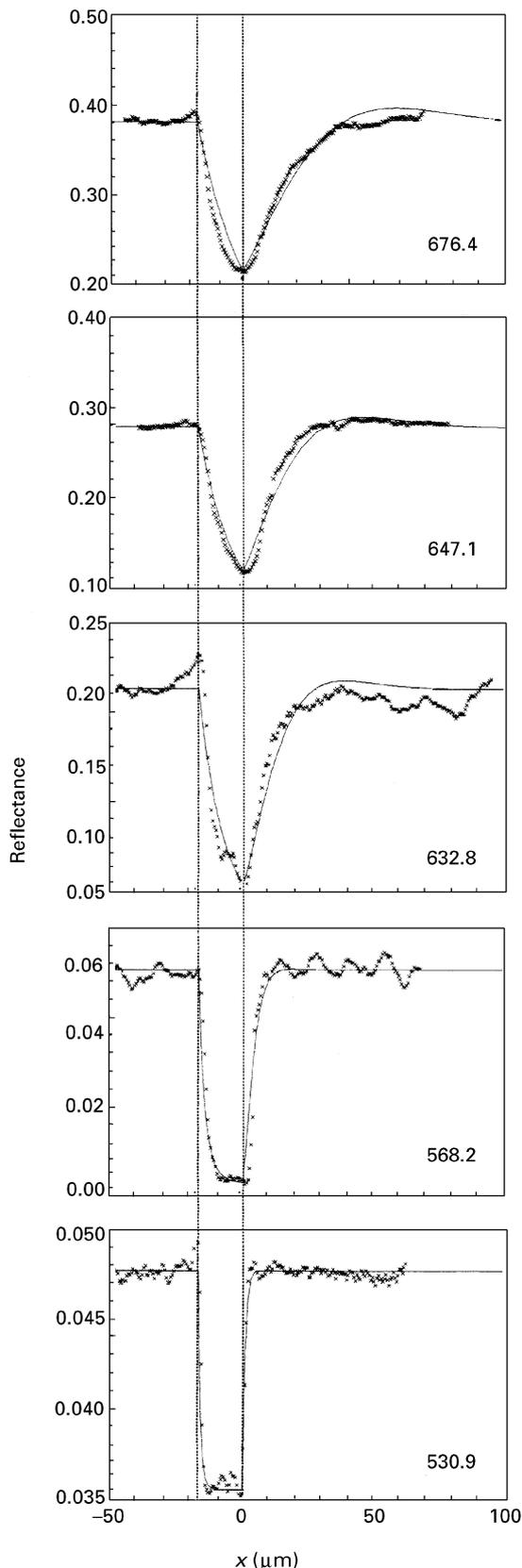
**Figure 9** Lateral resolution in SPR microscopy. The vertical lines denote the physical width of a 2.5 nm SiO<sub>2</sub> ridge. Number insets correspond to the various wavelengths used.
