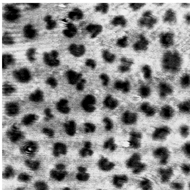
**Figure 8** SP microscopic image of an inhomogeneous monolayer. Dimensions of image  $0.2 \times 0.2 \text{ mm}^2$ . Thickness difference of the two types of domains is less than 0.4 nm. Lateral resolution approximately  $3 \mu\text{m}$ .
