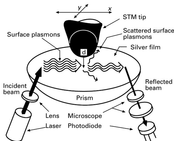
**Figure 12** Scheme of a combined SP microscope and a scanning probe microscope. The tip can either be a STM or an AFM tip. Reproduced with permission from Specht M (1992) *Physical Review Letters* **68**: 476–479. American Physical Society.
