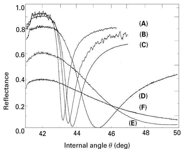
**Figure 2** SPR reflectance curves for a bare gold layer with thickness 44 nm, measured with different wavelengths: (A) 676 nm; (B) 647 nm; (C) 633 nm; (D) 568 nm; (E) 514 nm; (F) 488 nm.
