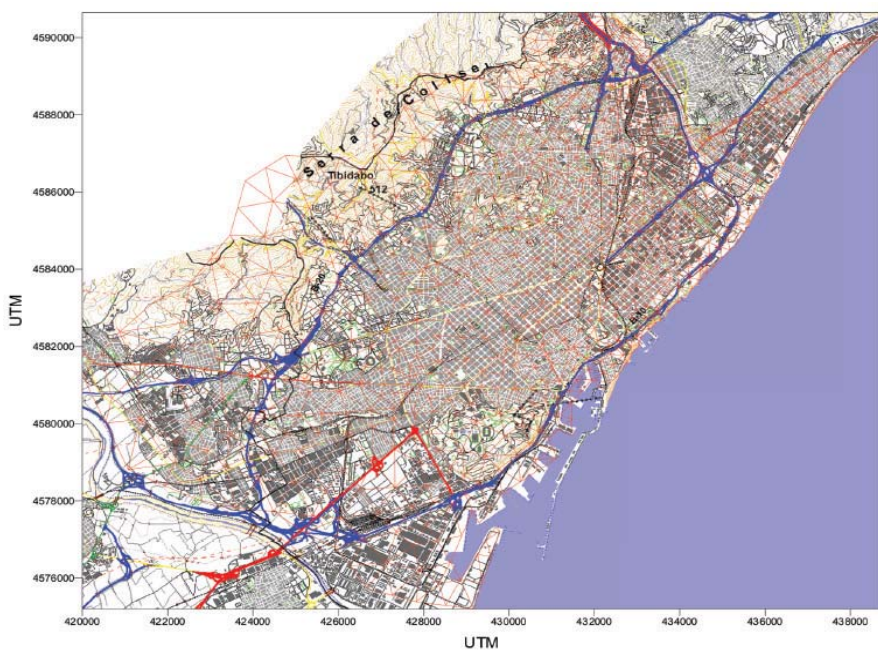
Fig. 4.1-2 Model domain, including street network (grey) and highways (blue), and finite element mesh (red)
