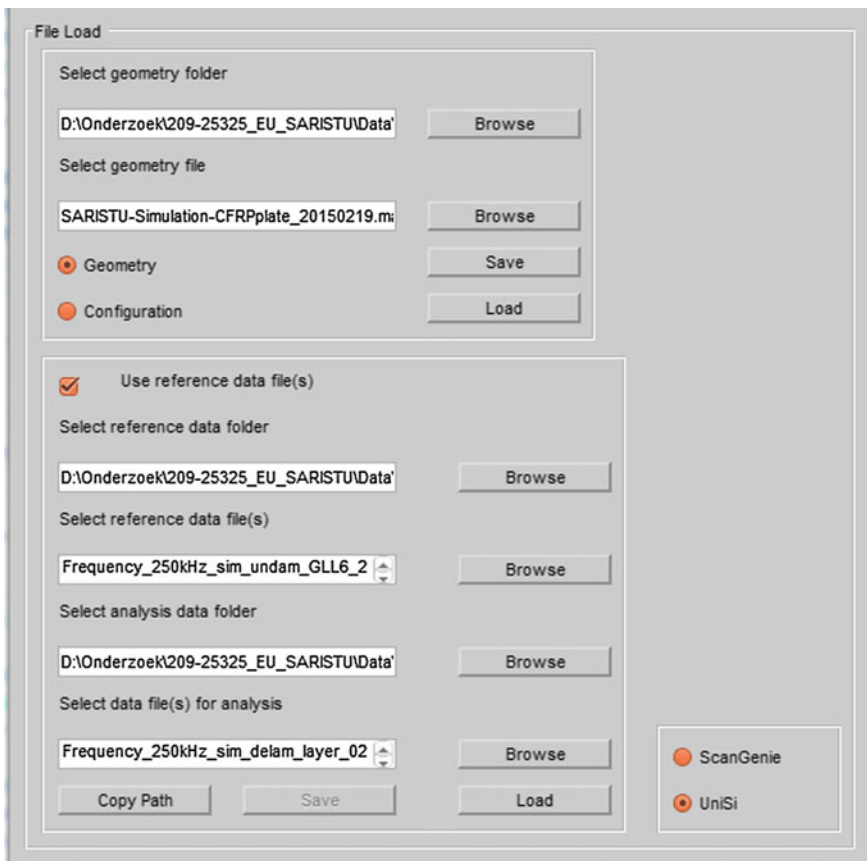
Fig. 3 File load panel. The file containing the geometric information is selected in the top part ; once loaded, the lower part of the panel becomes active and the signal data files can be specified and loaded
