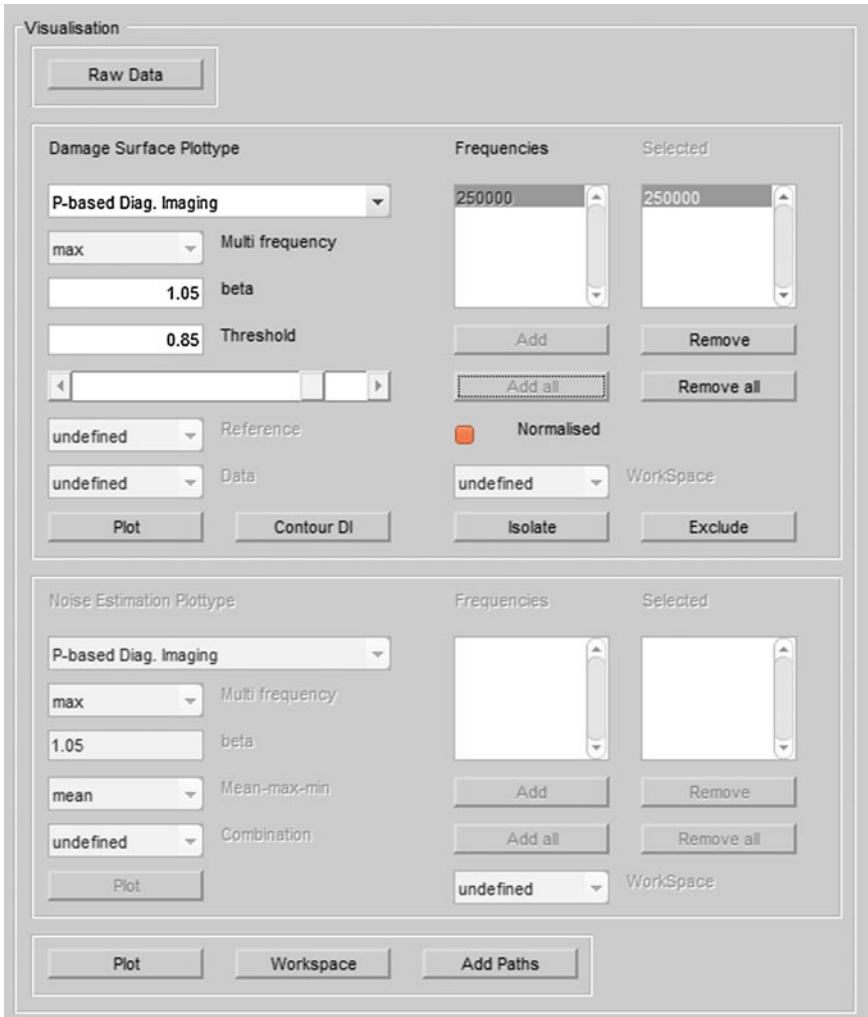
Fig. 6 Visualisation panel. This panel permits the user to control the graphical output displayed on the right-hand side of the GUI (not visible here)
