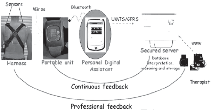
Fig. 47.2 Components, data transmission, and ways of feedback provision in the MYOTEL intervention. ( http://www.utwente.nl/ewi/bss/research/research_themes/macro/myotel_project/ )
