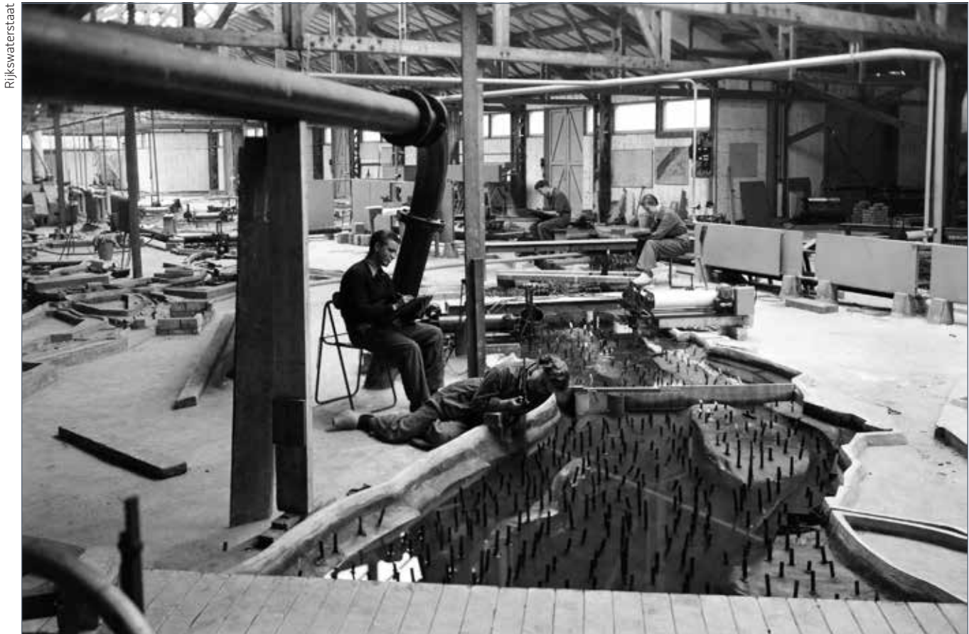
Delft Hydraulics Laboratory model of the southwestern delta, 1948–1956. This model has been used to simulate and predict tidal effects and water level changes during the construction of the Delta works. The Delft model was inspired by the lower Mississippi River model by WES in Vicksburg.
