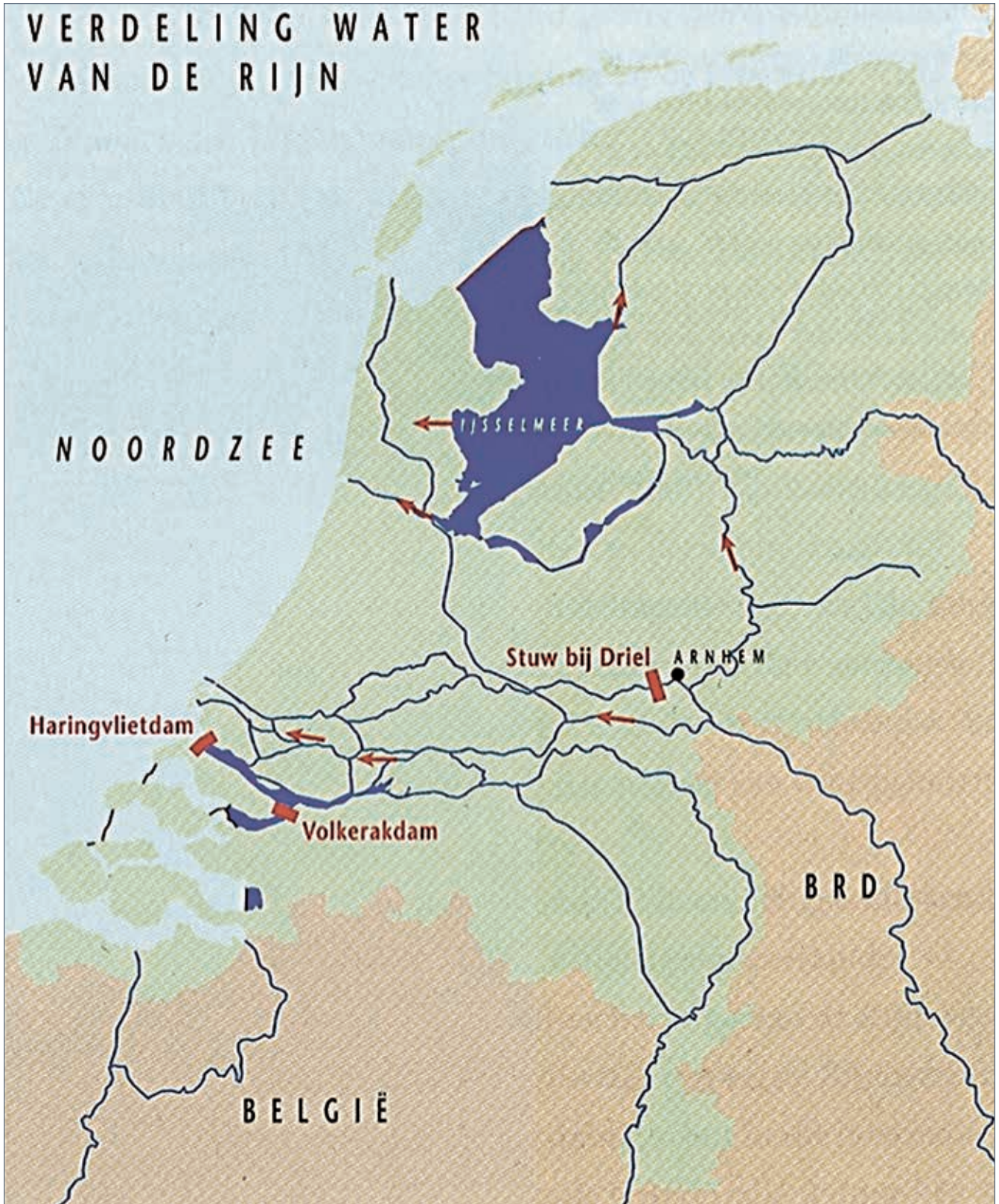
Nether-Rhine canalization system: at low Rhine stages, the Driel weir is closed to ensure fresh water flow to the IJsselmeer through the IJssel (upward arrow)
