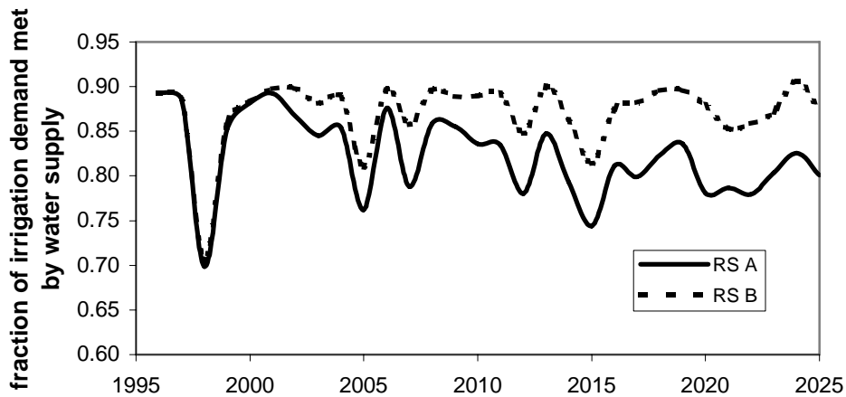
Fig. 6. Water supply sufficiency for irrigation: fraction of the water demand for irrigation that can be covered by water supply.
