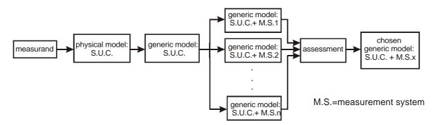
Figure 2. Sketch of the knowledge based system at top-level
