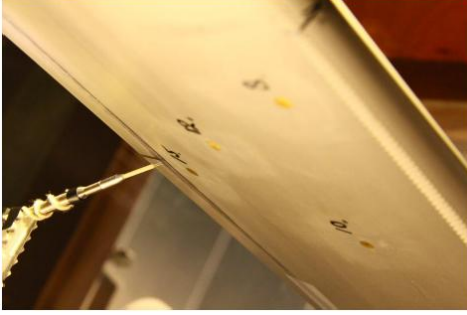
Fig. 9. Model with hot wire positioned above slit
