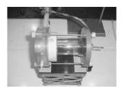
Figure 9: Custom  $\underline{}$  -made plasma reactor with nitrogen atmosphere by Hudec et al [17].
