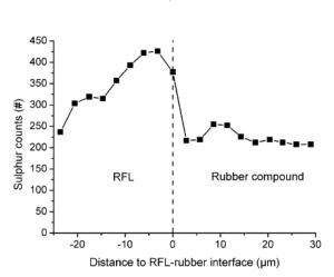
Figure 6: SEM-EDX linescan for sulphur of the RFL-rubber interface [7].
