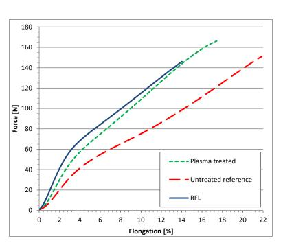
Figure 10: Effect of plasma treatment on Rayon cord in comparison to untreated Rayon cord and RFL dipped Rayon cord.
