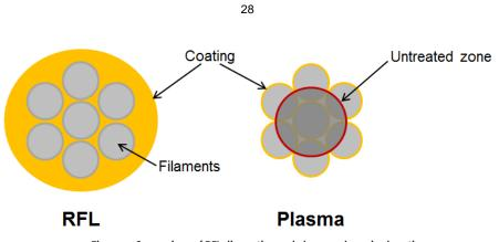
Figure 11: Comparison of RFL dip coating and plasma polymerized coating.
