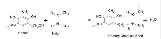
Figure 2: Reaction scheme of a resole and nylon molecule forming a covalent bond [6].
