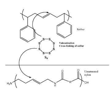
Figure 7: Crosslink reaction between rubber matrix and the innovative unsaturated nylon during vulcanization [10].
