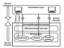
Figure 3: LMS model based on SOA reference architecture
