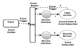
Figure 2: Event driven Architecture of 'Authentication Process'
