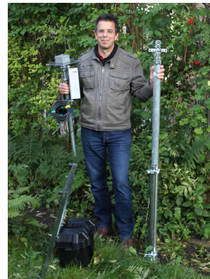
Fig. 10. The hybrid antenna-transmitter system can be made light and transportable. First author holds the top section of the mast with attached beacon transmitter (left) and the telescoping antenna mast (right). Mast foot and battery are shown at the bottom left of the picture.
