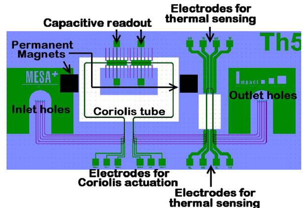
Figure 1. Structure of single chip flow sensing system.
