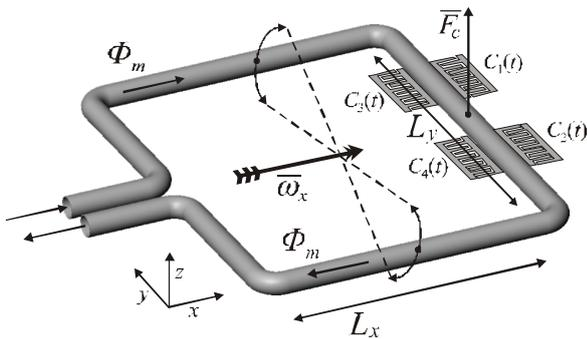
Figure 3: Coriolis flow sensor.
