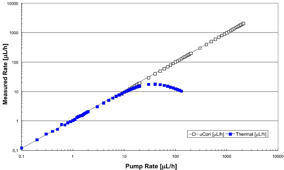
Figure 9. Measurement results demonstrating a dynamic range of more than 4 decades.
