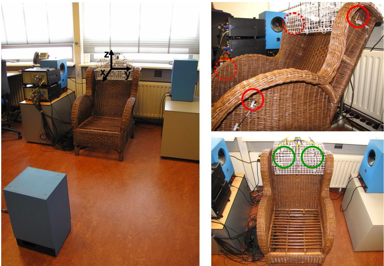
Figure 2. 'Silent Chair' experimental setup. The red circles show the physical locations, the green circles the virtual locations. The primary source is placed in front of the chair, the two secondary sources on the sides.
