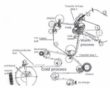
Figure 4. Processes and physical components performing them of a similar printer, taken from [2].
