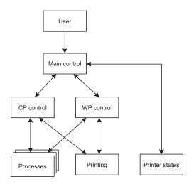
Figure 5. The high-level structure of the model describing the printer under different scheduling strategies.
