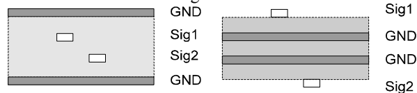
Figure 4: Cross-section of improved multilayer PCBs using the power isolation concept
