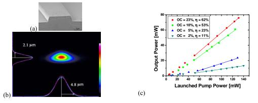
**Fig. 1.** (a) SEM micrograph of a microstructured KYW: $Gd^{3+}$ ,  $Lu^{3+}$ ,  $Yb^{3+}$  channel waveguide before overgrowth and (b) measured mode profile of the laser emission (both to scale); (c) measured output power as a function of launched pump power (approx. 99% of the launched pump power was absorbed) for different outcoupling (OC) values.
