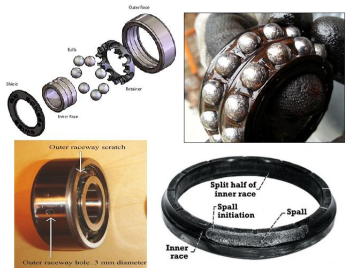
Fig. 2. Composition of a ball bearing (top left); damaged bearing balls (top right); outer race defects (bottom left); and inner race defects (bottom right)
