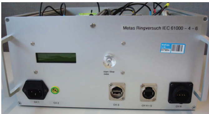
Figure 1. The front view of the conducted immunity round robin device
