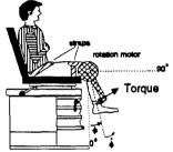
Fig. 1: Schematic of experimental set-up. Knee angle  $(\phi)$  and velocity  $(\dot{\phi})$  are defined positive in extension motion with zero as indicated. Subject is strapped at the hip and knee to measure knee torque (at the tibia) only and to ensure static position of the body.
