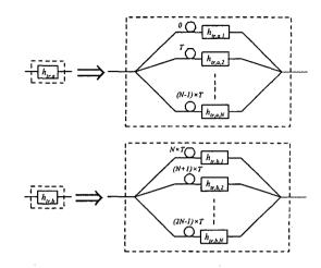
Figure 3: Substitution of transmitter filters
