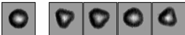
Figure 6 Mode vibrations for a Sonovue™ bubble with a diameter of 4 \mu\text{m} . Here a mode n = 3 is observed, however a range of modes is observed for a transmit frequency of 3.5 MHz.
