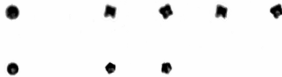
Figure 7. Mode n = 4 (top) and mode n = 5 (bottom) vibrations for small microbubbles of 1.4 \mu\text{m} diameter. The transmit frequency is 19 MHz. The images were recorded using a strobe technique on the Brandaris camera.
