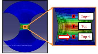
Figure 3; Schematic of elements selection for strain rate localization.
