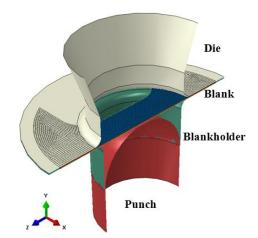
Figure 2; FEM Schematic of Nakazima test.
