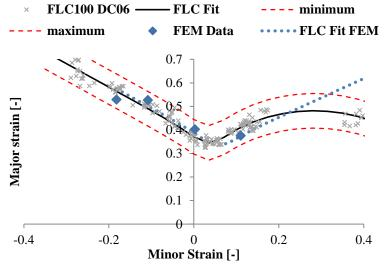
Figure 4; FLC experimental and FEM results for DC06 and 100 mm punch.
