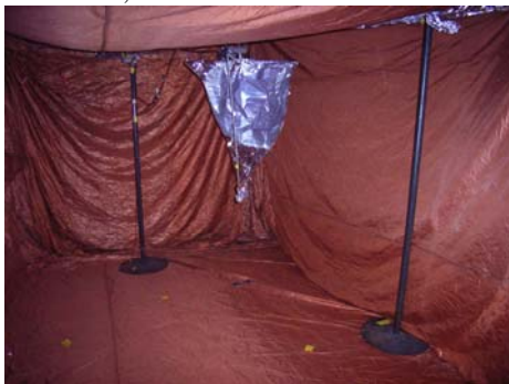
Figure 3: A Tuneable Intrinsic Reverberation Chamber, right outside, right inside
