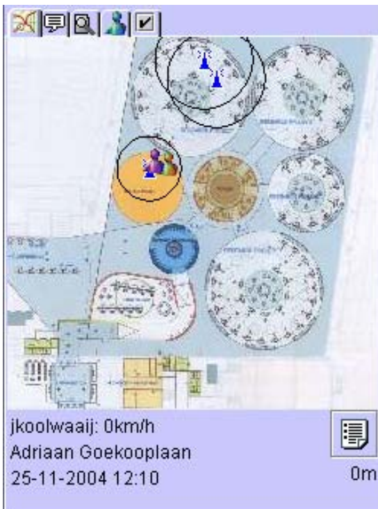
Figure 7. The situation after Ferdinand entered the train-station, coverage area of a public Wi-Fi hotspot. A seamless handover has taken place from GPRS to Wi-Fi, and based on that (network) context information the context reasoner has decided to switch from location provider as well.
