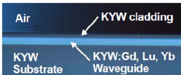
Fig 1. Microscope picture of the polished endface of the buried waveguide; white light was coupled in the waveguide for visualization.
