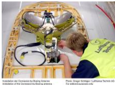
Figure 1 Installation mechanically steerable dish antenna
