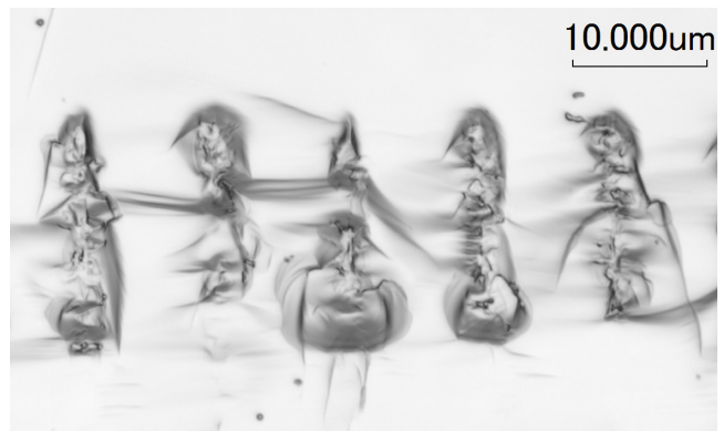
Figure 8: Laser scanning confocal microscopy intensity image of the sidewalls of the die after dicing, laser beam propagation direction: top-down. Wavelength: 1062nm, FWHM pulse duration: 170 ns, pulse energy: 5.2 \mu\text{J} , focus depth: 130 \mu\text{m} , M^2 : 1.1.
