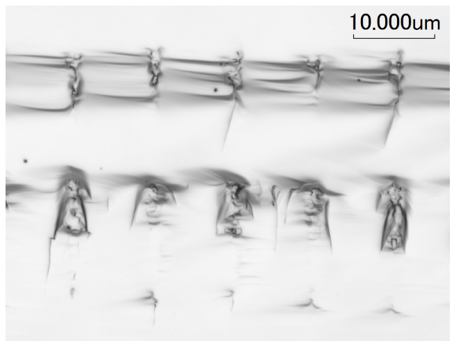
Figure 9: Laser scanning confocal microscopy intensity image of the sidewalls of the die after dicing, laser beam propagation direction: top-down. Wavelength: 1062nm, FWHM pulse duration: 170 ns, pulse energy: 9.35 \mu\text{J} , focus depth: 130 \mu\text{m} , M^2 : 1.1.
