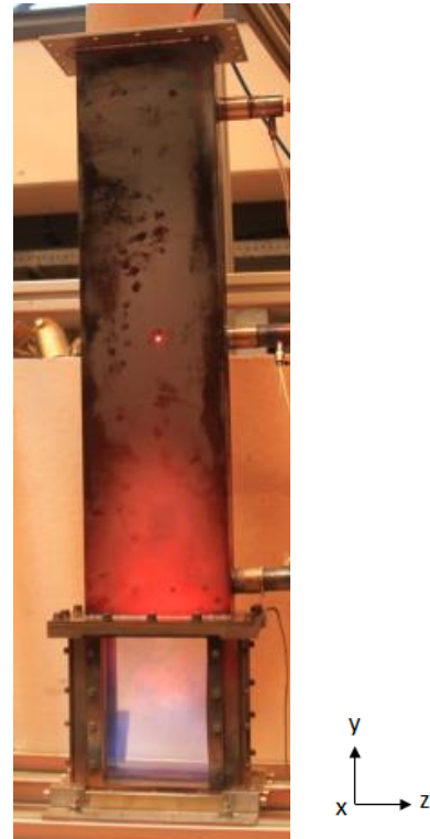
FIGURE 1: THE LIMOUSINE COMBUSTOR: THERMAL LOAD ON THE STRUCTURE IN AN UNSTABLE OPERATING CONDITION. RED DOT ON STRUCTURE CENTER IS THE LASER VIBROMETER BEAM
