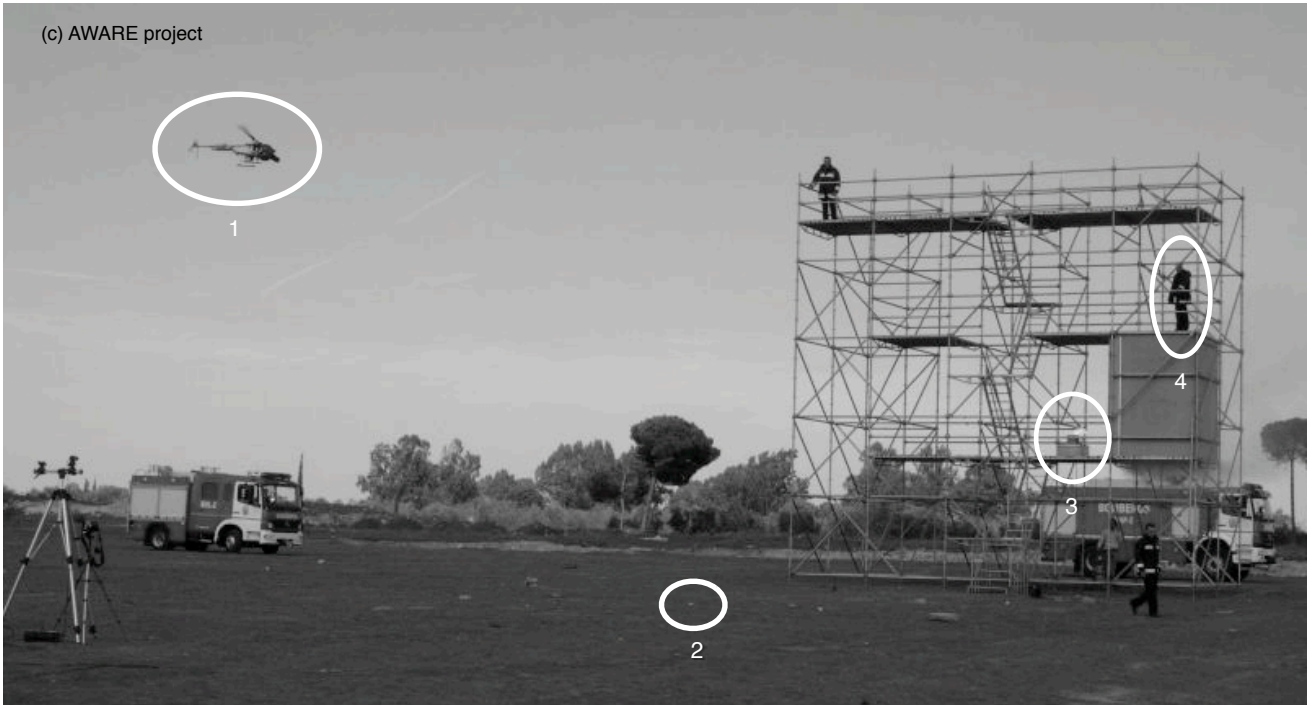
Fig. 1: Experiment setup. (1) Helicopter carrying a mobile node, (2) static node, (3) fire and smoke generators and (4) fire-fighter carrying a mobile node
