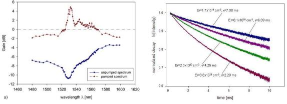
Fig. 1. Net gain in a sample with Er concentration 0.09at%  $(0.8 \times 10^{20} \text{ cm}^{-3})$  as a function of wavelength
