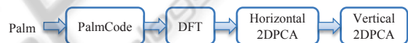
Figure 1: Flow chart of the proposed method. (DFT - discrete Fourier transform; 2DPCA - two-dimensional principle components analysis).
