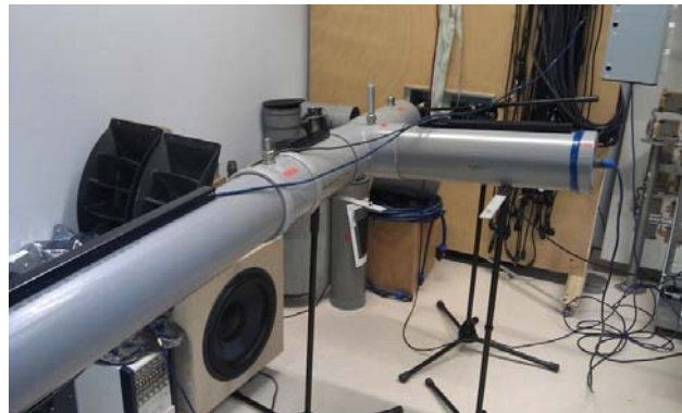
Figure 5: Experimental setup consisting of a duct for active noise control tests.
