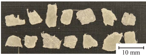
Fig. 2(a). Glass/TPU Type A flakes.
