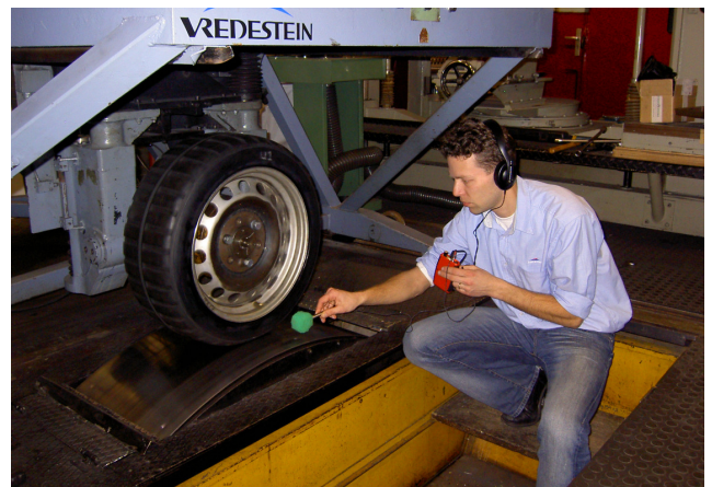
Figure 2: Tire -drum measurement set-up.
