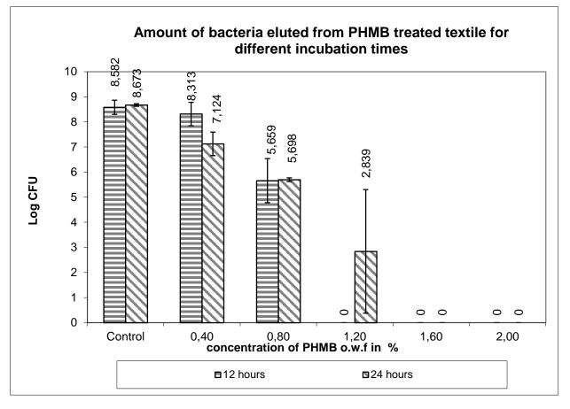
Figure 1. Amount of bacteria eluted against concentration of PHMB o.w.f in % for different incubation times
