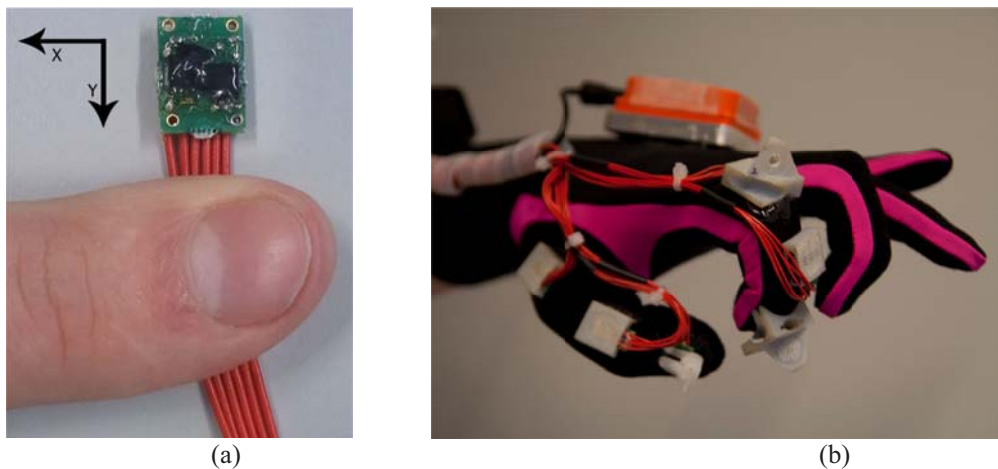
Figure 4. (a) first version of a movement sensor PCB with 3D accelerometer and magnetometer, (b) the first prototype kinematic glove with partial instrumentation of index finger and thumb [4]
