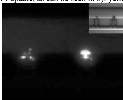
Figure 3. Fluorescence image of cells located at the traps and being electroporated and loaded with green fluorescent nanobeads ( 60\text{nm} ). Right top, light image of the cells.
