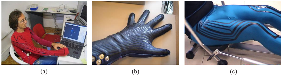
Figure 2. Fabric-based human motion monitoring devices using screen printed piezoresistive rubber sensors and sensor track (black stripes in the garments), developed by the University of Pisa and Smartex [5]: a) upper-limb monitoring device developed for post stroke telerehabilitation. b) instrumented glove. c) fabric-based motion classification garments for monitoring leg kinematics.
