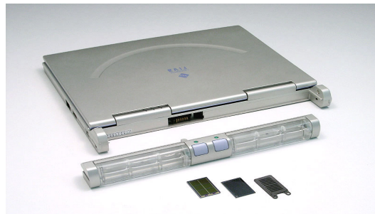
Figure 4. Prototype of a laptop with Direct Methanol Fuel Cells (DMFC) of Casio
