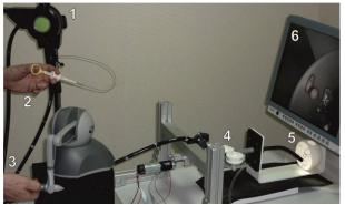
**Fig. 1** Robotic control flexible endoscope: (1) Traditional endoscope with driving means for tip steering, (2) Manual instrument control (3) Multi-DOF controller for tip steering and shaft control, (4) Driving means for shaft actuation, (5) Training model, (6) Monitor.
