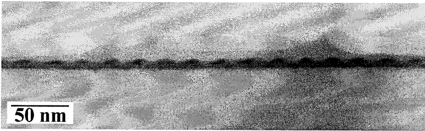
Figure 3. Cross sectional TEM of a thin film of IF 36/12 after O_2 -RIE treatment. The Fe-Si-oxide domains appear dark in the TEM, as does the silicon oxide layer at the surface of the silicon substrate.
