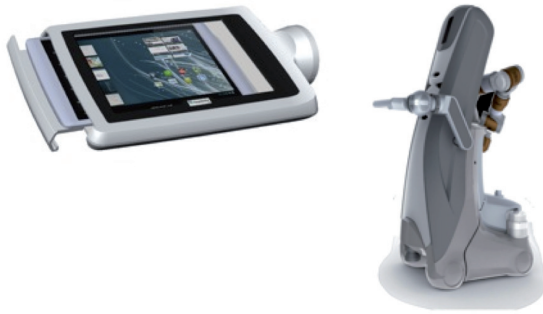
Fig. 6. Design drawings of the new tray kinematics with 3 degrees of freedom that allows height adjustment of the tray and switching between tablet pc and object placement
