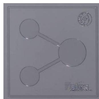
Figure 2: Picture of a microfluidic system made from PDMS, to be bonded on a glass substrate.
