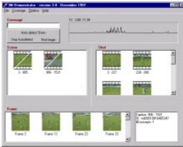
Fig. 7. User interface of the SVRS annotation module, the upper right window shows the color histogram of the current frame.
