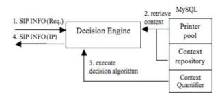
**Fig. 3.** Handling of printing requests in the decision module of the context broker. An incoming request triggers the execution of the decision algorithm, which in turn uses information stored in the database to select a PPS. Subsequently, it sends a response with the PPS's IP address to the requestor. Responses and requests are carried as SIP INFO payloads.
