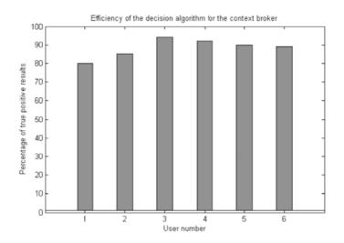
**Fig. 6.** Efficiency of the decision algorithm in the Context Broker. Efficiency is determined by the percentage of correct results from the algorithm (i.e. true positive outcome)
