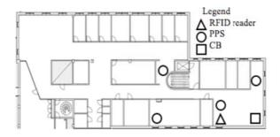
**Fig. 1.** Deployed system topology. A context broker ("CB") acts as a repository of context information coming from Printing Point Services – "PPS" (printer status and capabilities), as well as RFID readers – "R" (user location). The CB is also responsible for handling printing requests from mobile users by designating suitable a suitable printer.
