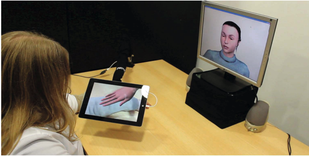
Fig. 1. The components of the TVA setup. The monitor displays the agent's upper body, allowing the agent to gaze at, and talk to the user, as well as show body movements in accordance with the touch. The tablet computer displays the agent's hand touching the user. The user wears a vibrotactile sleeve to generate a tactile sensation in accordance with the agent's touch.
