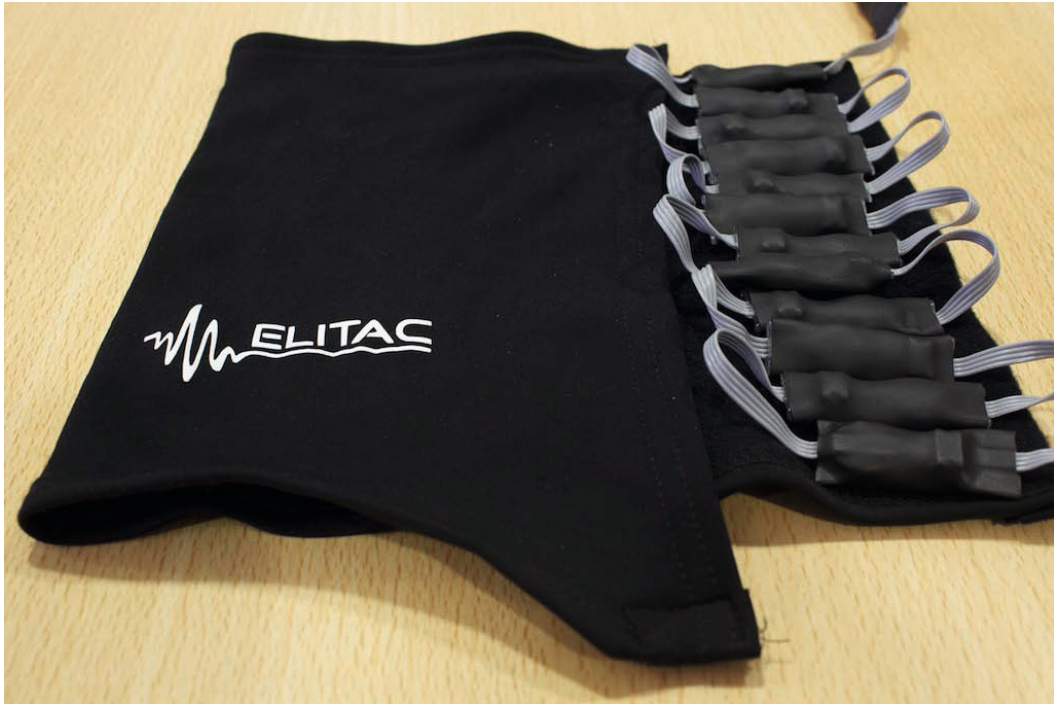
Fig. 3. The vibrotactile sleeve with 12 vibrationmotors
