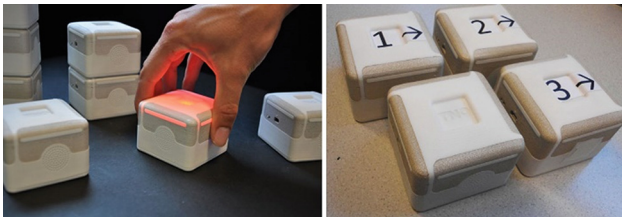
Fig. 1. The Sensors. The grey areas are coated with conductive paint and are connected with touch sensors. Left: activated Sensor emitting red light. Right: numbers on top serve to identify the Sensors. Arrows serve to indicate their orientation.
