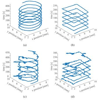
Fig. 4. Representative closed-loop motion control experimental results. Both trajectories are centered in (6 mm; 6 mm) with respect to the coordinates in the graph. In *a*) and *b*) the system operates in nominal conditions. In *c*) and *d*) an impulse-like disturbance is introduced every 3 s.
